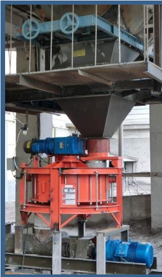
Rotor weight feeder with capacity up to 40 t / h and precision control of 0.5%
